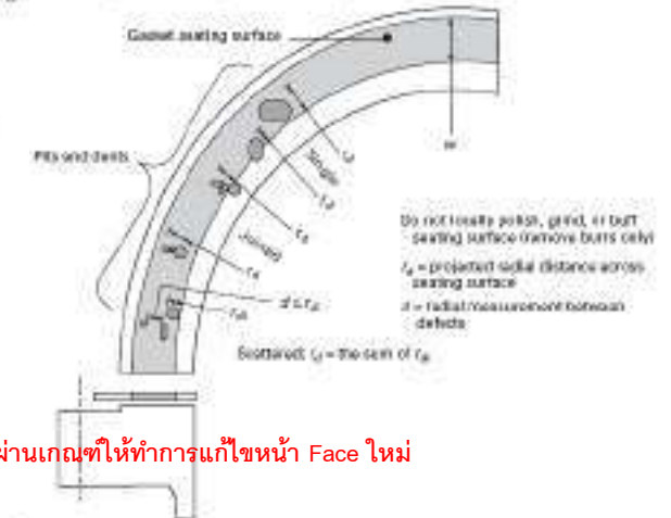
Fig. D-3 Flange Surface Damage Assessment: Pits and Dents
